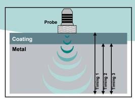
small echoes gives us the timing of the echoes within the metal, which relate to the metal thickness. The returned echoes need not be consecutive as the gauge will interpret them automatically and calculate the thickness. A minimum of three echoes are checked each time. This is referred to as the **Automatic Measurement Verification System (AMVS)**.
